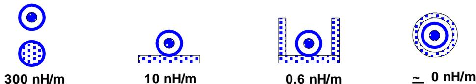
Figure 1: Shapes of parallel earthing conductors and their effect on transfer impedance.
