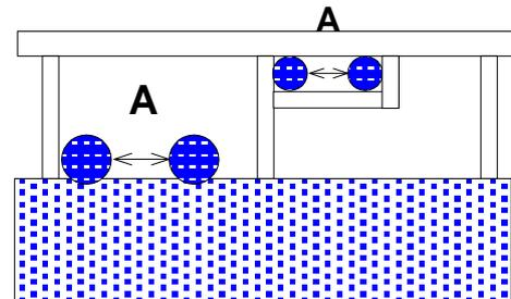
Figure 2: The distance between the cable and the fluorescent, neon or high-density discharge fixtures shall be at least 130mm.
