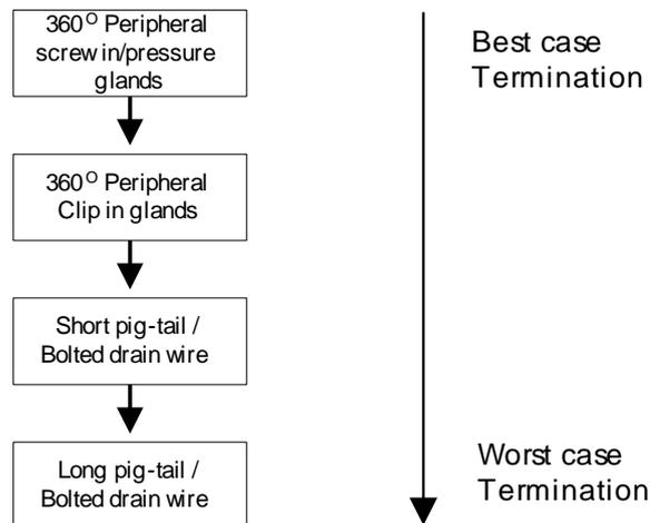
Figure 3: Best to worse case cable screen termination
