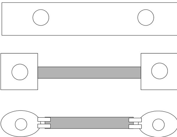
**Figure 4: Examples of Bonding straps**
